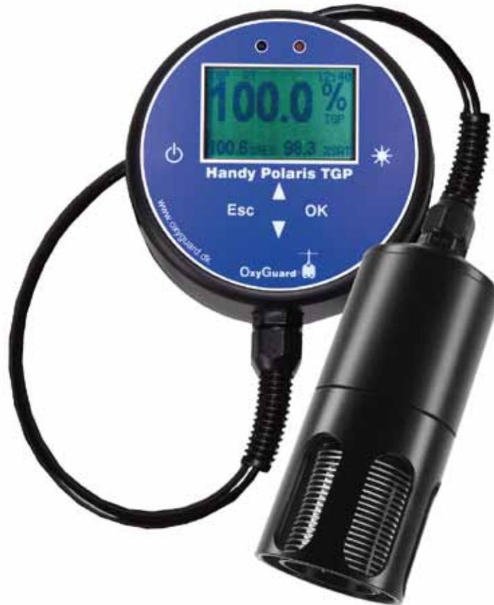
The OxyGuard Handy Polaris TGP is a hand-held gas pressure meter. It can operate in three modes, one where it acts as a standard Polaris dissolved oxygen meter, one where it is a Total Gas Pressure meter that shows pressures as “percent saturation” values of the actual atmospheric pressure and one where it is a Total Gas Pressure meter that shows pressures as volume percentages.
