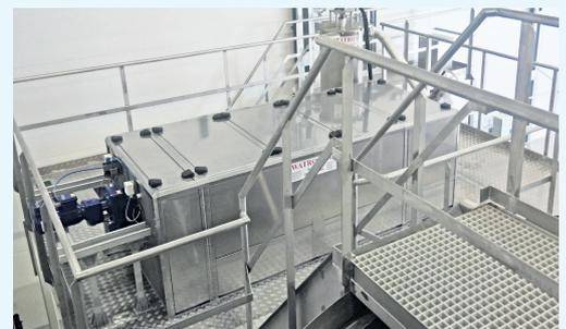
The sludge treatment (MDD-process) has been developed for dewatering and drying of the sludge fraction from effluent treatment in aquaculture. Gas production has been successfully adapted on the basis of sludge, directly from water effluent filtration.
